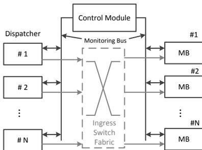
Fig. 3. Connection among Dispatchers, MBs and Control Module
