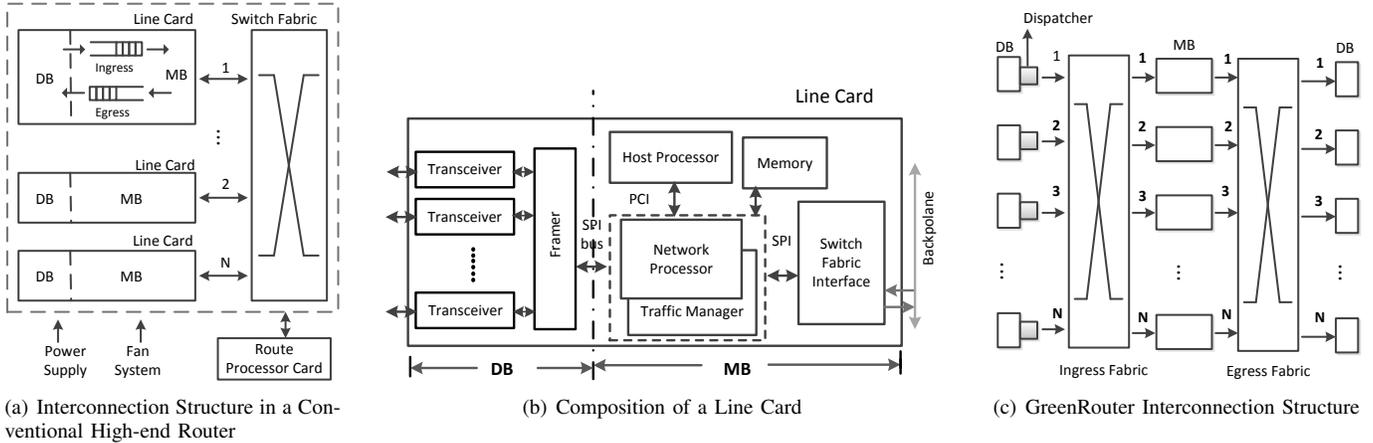
Fig. 2. Architectural Comparison between the Conventional Router and GreenRouter
