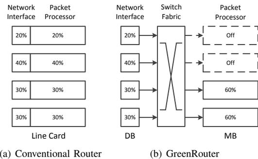
Fig. 1. An Illustration of Power-proportionality Comparison
