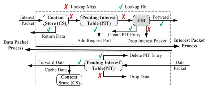
Fig. 1. Packet Forwarding Process in an NDN Router
