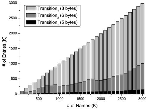
Fig. 7. Number of Entries for Transition<sub>1</sub>, Transition<sub>2</sub> and Transition<sub>4</sub> on DMOZ dataset
